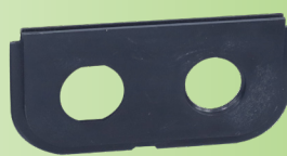
One dia 21 x 19.6mm hole for M21x1 connector and one M20x1.5 for cable gland.
