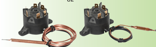
3 pole manual reset high limit thermostat, fail safe, fixed setting, temperature range up to 170°C
